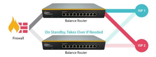
When your organization has a corporate requirement demanding the highest availability with no single point of failure, you can deploy two Peplink routers in **High Availability mode** (http://www.peplink.com/knowledgebase/configuring-11-backup-by-vrrp/). With High Availability mode, the second device will take over when needed.
